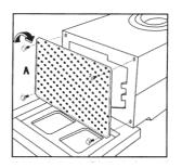
4. Unscrew and remove the four feet. Fit the grid on the bottom of the machine and re-fit the four feet. Tighten up the lock nuts on all feet.
